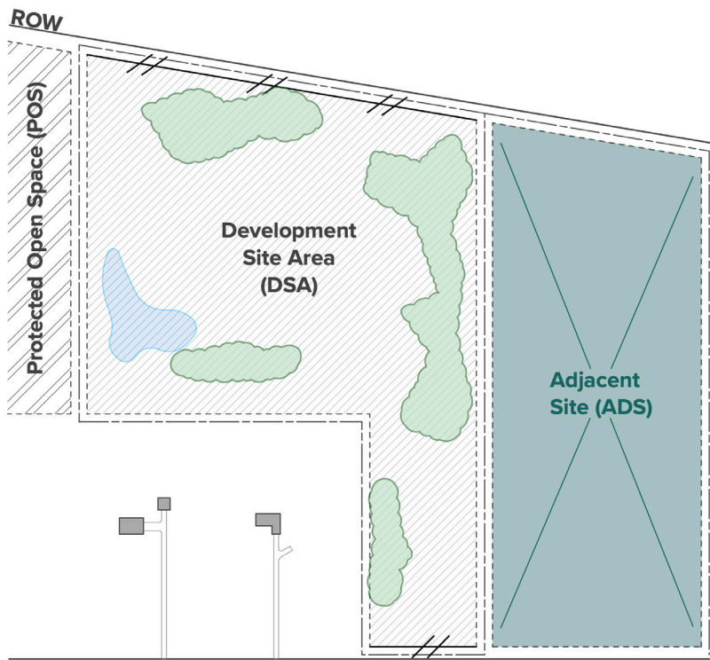
Existing Conditions Diagram (Above): Illustrate extent and context of the development site including existing woodlands, rivers/streams, and/or wetlands. Aerial Photos of site with property line are acceptable. Diagram NTS.
