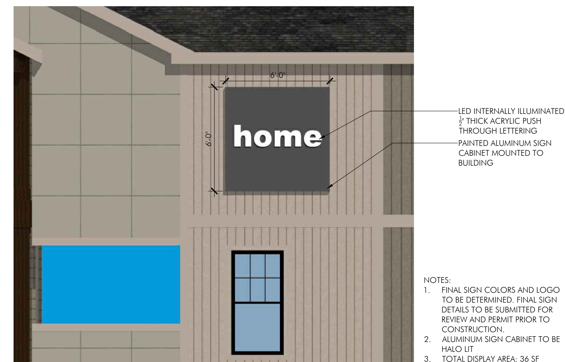
3 Building D Sign Detail SCALE: NTS
