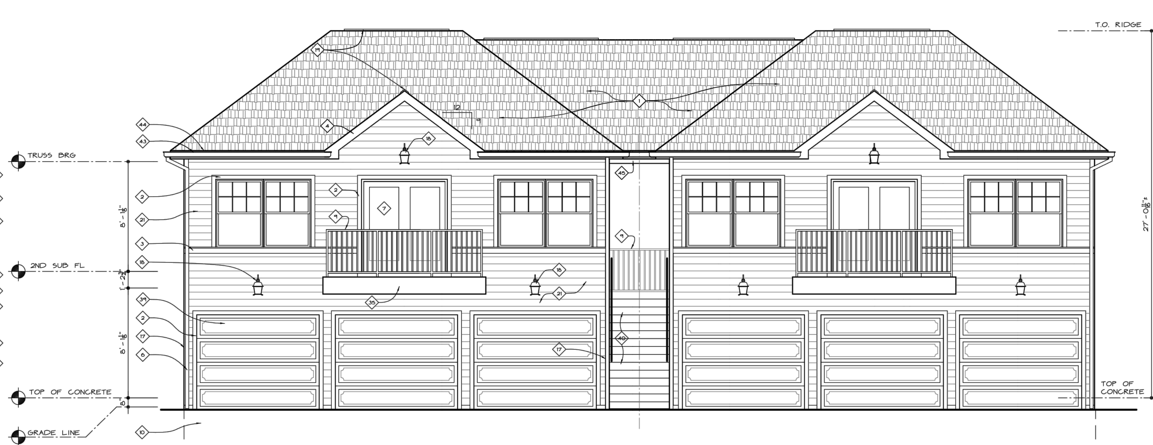
SF-CARRIAGE HOUSE FRONT ELEVATION - BLDG. TYPE 3 1/4"=1'-0"
