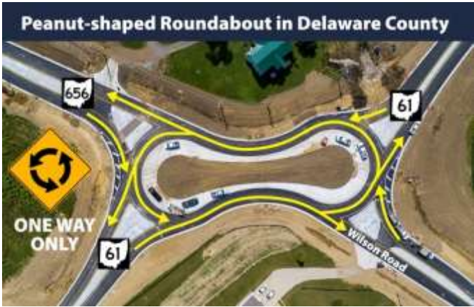
ODOT completed construction of a peanut-shaped roundabout at the intersection of State Route 61 and SR 656/Wilson Road. In addition to reducing crashes by 70 percent, the safety upgrade is expected to improve traffic flow at the intersection. The $2 million safety project began in May 2021 and opened to traffic Monday, August 9, 2021.
