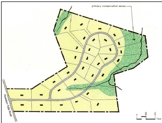
Traditional subdivision of large lots, leaving no common open space – Yield Plan
