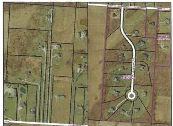
(left) “No Plat” Lot splits in Berkshire where all lots have frontage on an existing road. (right) Hickory Woods in Genoa Township, a conventional subdivision with large lots.
