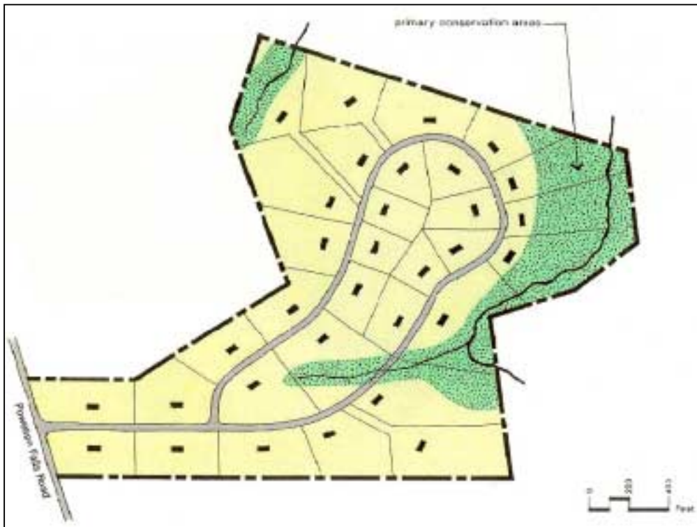
Traditional subdivision of large lots, leaving no common open space – Yield Plan
