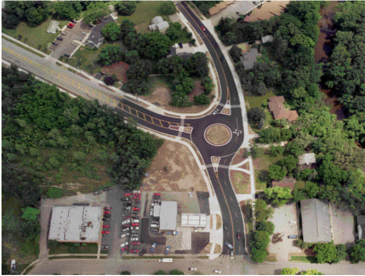
Figure 4G Example of a Modern, Low-Speed Roundabout
