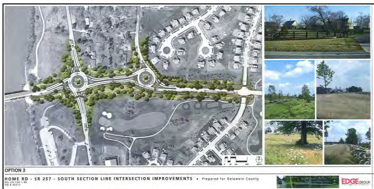
Drawings for the now complete South Section Line/Riverside Drive/Home Road double roundabout.
