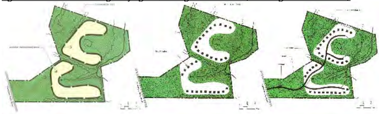
Figure 13c. Conservation design: Laying out building sites and roads (according to Randall Arendt)
